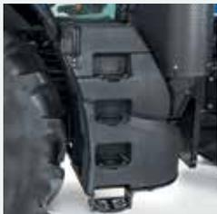
Right hand steps to assist in cleaning right door window to improve visibility when working.
