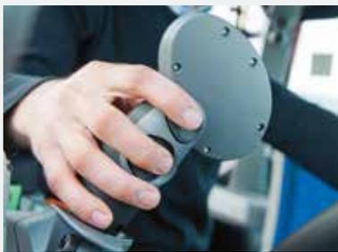
The button on the rear of the CommandGrip™ gives access to further functions.
