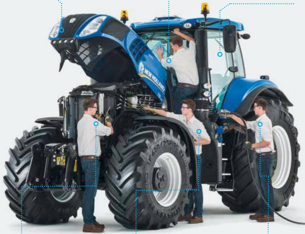
Cooling package opens out to make cleaning faster and easier.
