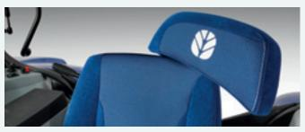
Both the Dynamic Comfort and Comfort seats benefit from an innovative swivelling backrest, designed to provide upper back support and significantly increases comfort when the seat is turned to monitor rear mounted implements.
