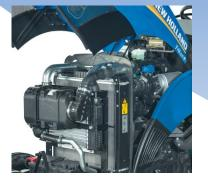
The engine air filter is easy to check, clean or replace, with no need for tools.
