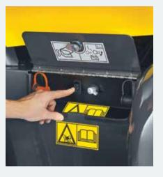
• Hood switch, kill switch and remote battery terminals are grouped at the rear
