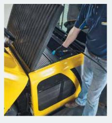
• Easy access to each of the individual radiators allows easy routine cleaning
