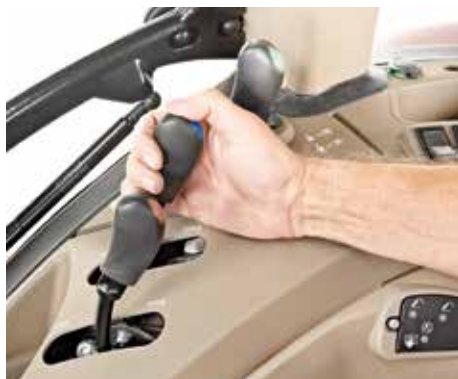
Up to three mechanical rear remote valves are available for the Farmall C range.
