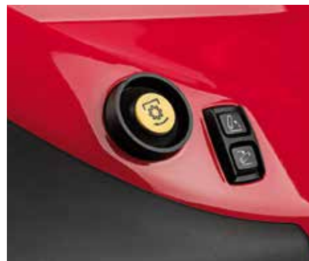
External controls for fast and easy implement attachment on EHC tractors.
